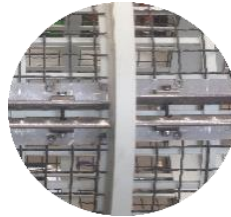
Additional internal wire screens optional 40 to 80 mm
