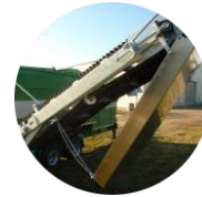
Permanent drum magnet with slide
